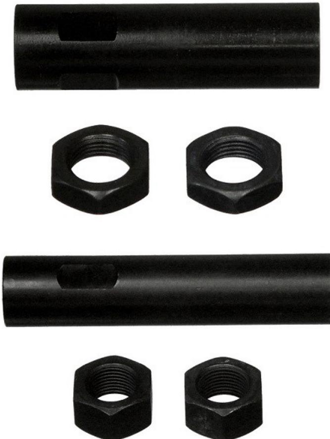
These sleeves are what makes these ordinary parts so much stronger than the stock ones. These solid sleeves are available off the shelf from MOOG one is ES3201S which measures out at 3.35" end to end and will cover Amigo 1988-1994, 4WD pickup 1988-1995, Rodeo 1991-1995, Trooper 1987-1991. All of these application will require cutting off 7/8" from the male threads on the tie rod end to make them shorter so they don't bottom out against each other
