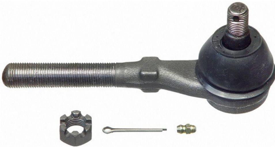
Above is Moog ES3369T and ES3370T which upgrades the rod thread to 18mm but keeps the same stud thread and taper so it will bolt up to the stock knuckle.
