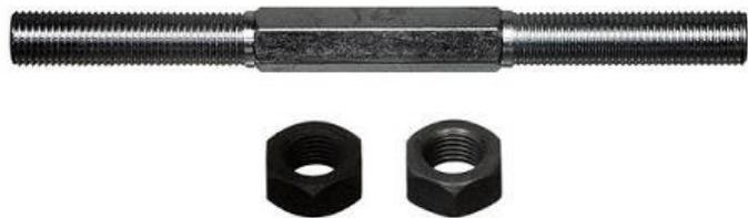
**Above you will see the only two adjuster rods sold by MOOG for the Isuzu. The longer one on the top ES3089S measures 8.42" from end to end and is listed for 2WD Isuzu Pickup Trucks. The shorter one on the bottom ES3090S measures 6.63" from end to end and is listed for Amigo 1988-1994, 4WD pickup 1988-1995, Rodeo 1991-1995, Trooper 1987-1991.**
