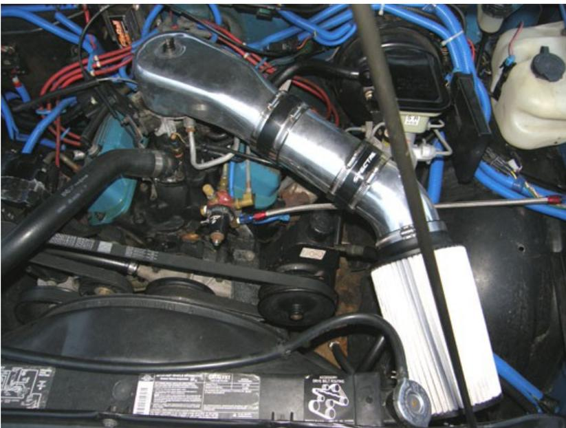
Here is the cold air intake unit installed on a 1993 S-10 with a 2.8L. Any S-10 with a 4.3L would be an almost identical install and can use the same parts.
