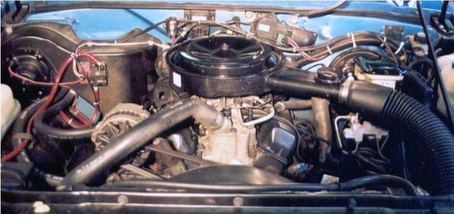
**The typical stock air cleaner on a GM TBI equipped vehicle. This is a Chevrolet S-10 2.8L**
