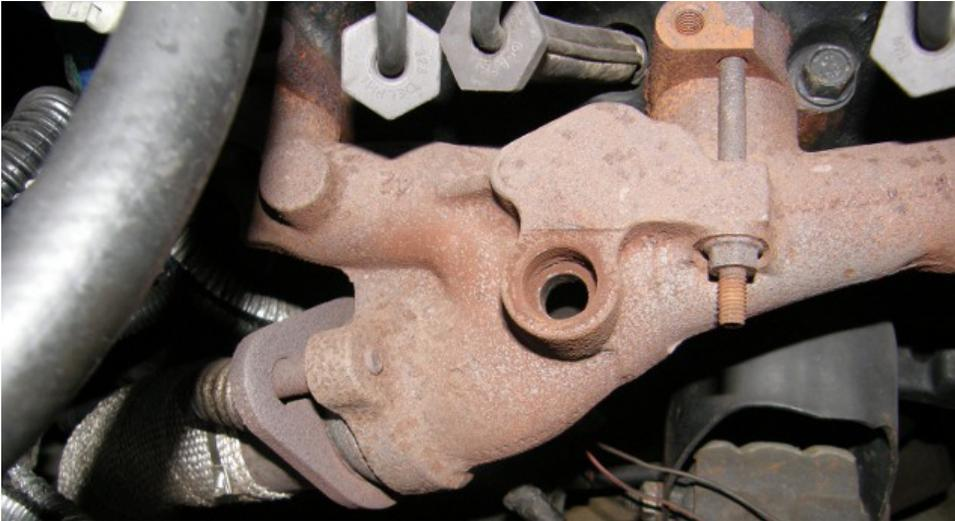
**This is the hole in the exhaust that needs to be plugged. The threads are 7/8-18 and can be plugged with an oil pan bolt or a male SAE Inverted Flare Plug.**
