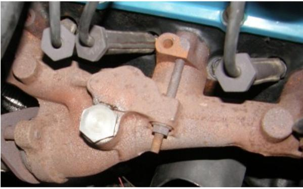
**Here is the plug and washer installed into the manifold. Make sure you clean up the rust build up on the surface where the washer seals against. Also if you need a tap to clean the threads it may be easier to tell the parts person you need to repair a 7/8-18 spark plug thread. Snap-On sells one as part number T2818 and it runs around \$25. Just make sure you vacuum out any filings that drop down.**
