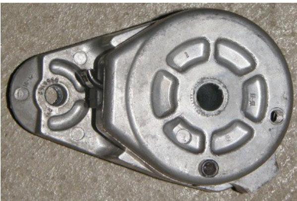
**Here is the back of the tensioner. This is an aftermarket replacement for a stock 2.8L. Notice the old pin position at the right. It was relocated by drilling and tapping the aluminum casting. The pin is 90 degrees to the pulley. The pin is a 1/4UNC Allen head cap screw.**
