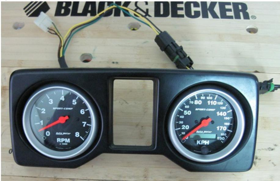
**Here are the gauges installed in the stock instrument panel cover. No modifications are needed which makes this such an inviting swap.**
