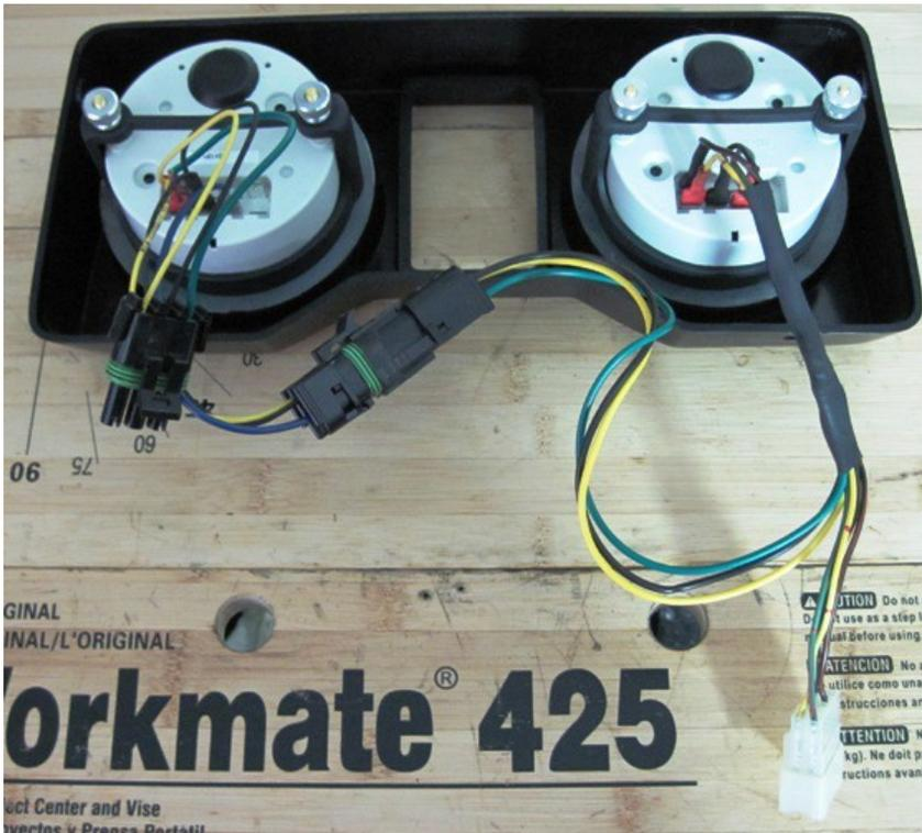
Here is how the wiring will look when completed. The black connector on the left attaches to the new VSS wiring. The black connector in the middle goes behind the divider in the dash and the white connector on the lower right is stock tachometer plug. You can see the reinforcement rings made to provide a more solid mount for the gauge retainer. The rings are 3 3/8" ID x 4 1/8" OD 10gauge steel.
