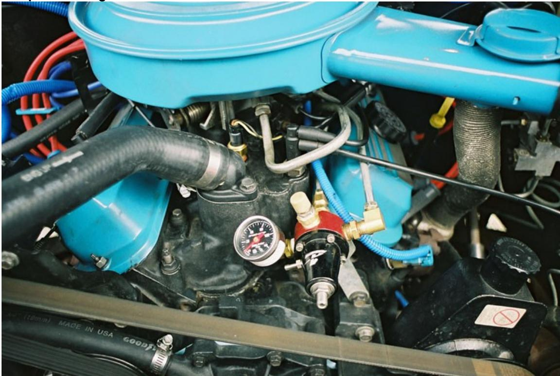
Now that you have completed either one of these modifications you can now start you engine and check for leaks. There is also a fuel pump prime lead which is a gray wire with a black connector on it. By giving this connector positive power you can run you fuel pump and check for leaks. Leaks will commonly occur at the diaphragm/gasket of the stock regulator. So be sure you check under your air filter lid.
