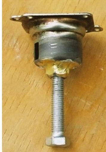
**You can see how an adjustable fuel pressure regulator is made. There is a nut welded on the end where the bolt threads through. This bolt will move the spring retainer up or down and allow for adjustable pressure.**
